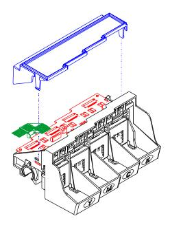
Figure 5-3. Electronics Cover Removal.
